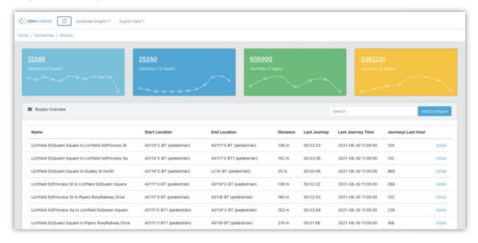
As a traffic management tool, **Senseview** collects and collates data from tracking journeys through a combination of video image and unique user digital signature in vehicles as they pass through detection points.
